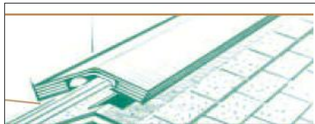
Figure 68 details an example of the “Trimline” ridge vent profile installed over the roof ridge.
